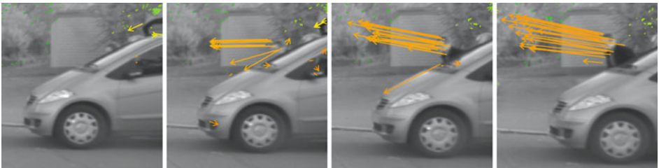
■ Fig. 29.7 Estimation result of the 6D-Vision algorithm for the moving, partially occluded pedestrian after 0, 80, 120, and 240 ms from first visibility
