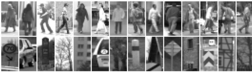
Fig. 4. Pedestrian and nonpedestrian samples from the benchmark data set (upper versus lower row, respectively).
